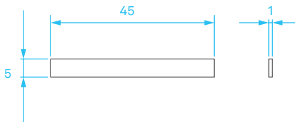
Marking Inlay for (64x64) mm →
