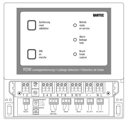
The contact overviews shown for the "break" and "alarm" relays under terminal assignment in the documentation for the connected RDW 03 are depicted with the following status:
