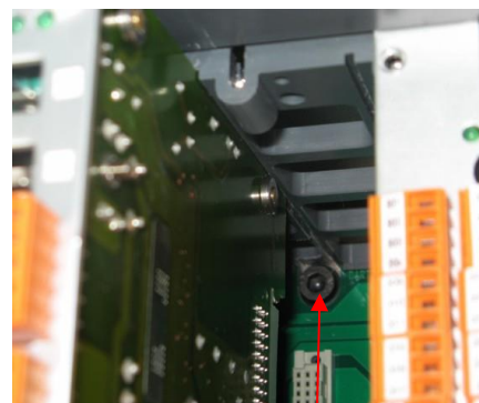
Mounting screw 4 Below module slot 1xx (the power supply unit must be removed to release it.)
