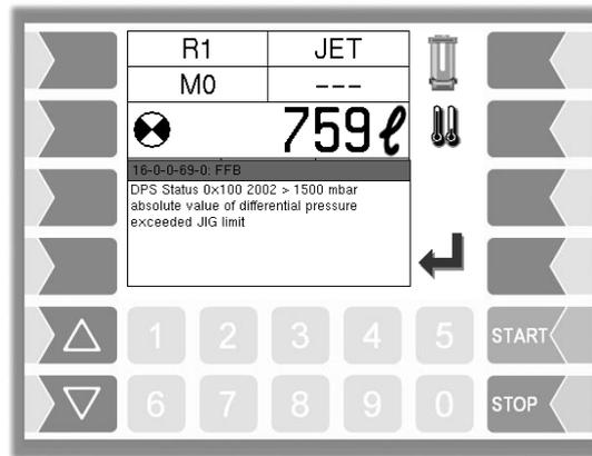
You can lock off the dispensing barrier, when the cause for the differential pressure exceeding has been eliminated (e.g. by filter replacement).
