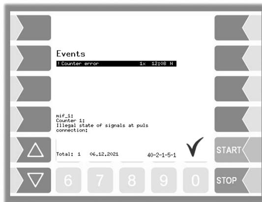
If an error occurs which prohibits a measured delivery, the pump will be disabled. The delivery must be finished.
