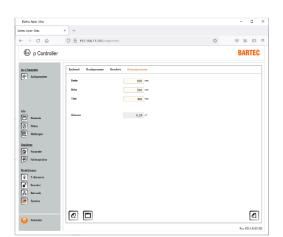
The internal volume of the pressurized equipment is defined in the " Enclosure parameters" tab.
