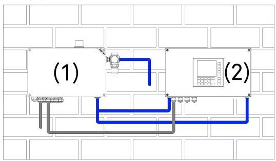
The typical arrangement is remote mounting, e.g. wall mounting, with a maximum distance of 5 m and an inner diameter of at least 10 mm between Ex p control unit and protected equipment.
