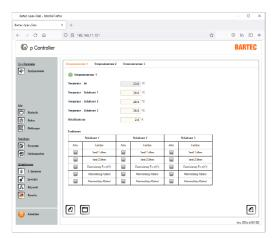
In the menu "T. sensors" up to three PT100/1000 sensors can be configured.
