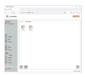
Within the "Save / Parameters" menu, parameters from the Ex p control unit can be saved on a local computer or transferred from the local computer to the Ex p control unit.
