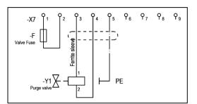
The terminal row X7 is used to connect the purge gas valve and the accompanying valve fuse. Furthermore, the terminal points 6 – 9 are intended for unused wires of the LAN connection cable.
