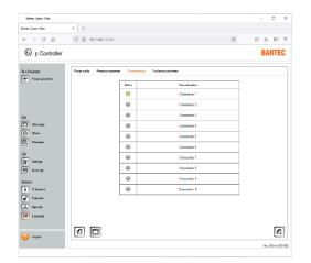
For automatic purge time determination, the characteristics of the pressure switch in the system must be set in the Ex p control unit.
