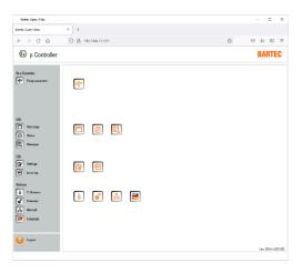
By clicking on the left-hand grey navigation bar, you can jump directly to specific submenus.
