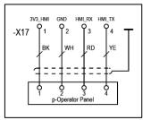
The optionally available p operator panel can be connected to the terminal row "X17".
