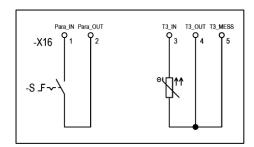
The BARTEC parameter-setting switch must be used to change the parameters.
