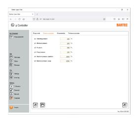
po = Operating pressure. Pressure value at which control takes place during the operating phase.
