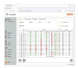
Manuel / Automatic = Determines whether the Ex p control unit performs purging with a fixed stored or automatically determined purge time.
