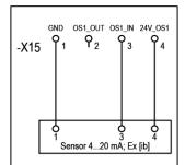
Pressure or gas sensors with 4...20 mA output can be connected to the sensor input OS 1 [Ex ib].
