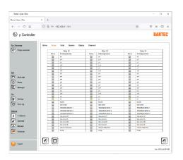
In the "Relay" menu item, the relays K2, K3 and K4 can be provided with the associated switching functions. One or more switching functions can be assigned to each relay.
