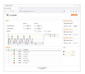
The start screen provides an initial overview of the status of the Ex p system.
