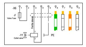
The terminal row X6 is used to connect the outlet valve and the accompanying valve fuse. Furthermore, the terminal points 6 – 9 are intended for the LAN connection cable.
