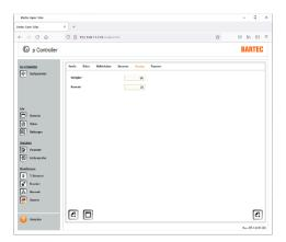
In the Display tab, the contrast and brightness of the LCD display can be set on the p-Operator Panel.
