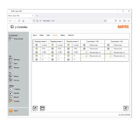
In the menu item "Sensors" the three additional temperature sensors can be activated.
