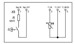
For the bypass switch to be detected and the function to be executed, a resistor with 620  $\Omega$  must be connected to the closing contact.
