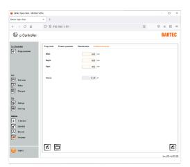
For automatic purge time determination, the size of the protected volume must be set in the Ex p control unit.
