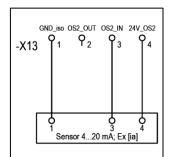
Pressure or gas sensors with 4...20 mA output can be connected to the sensor input OS 2 [Ex ia].
