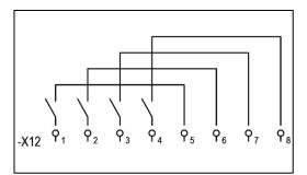
A floating signal (4x NO) is available on the Ex p control unit. This signal can either be used as an enable that is also safety related.
