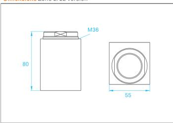
The pressure monitor module forms part of pressurised enclosure control systems. Various versions are available for applications in Zones 1/21 and 2/22.
