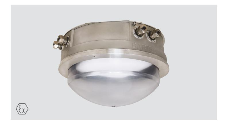
The EXgate<sup>™</sup> 360 enclosure makes it easy to deploy any wireless network in hazardous areas, Zone 1/21. The EXgate<sup>™</sup> enclosure can be used for all types of Wi-Fi, BLE, 4G/5G access points, radios, gateways and repeaters with internal and/or external antennas. All common connection standards are supported such as POE and Fiber optics.
