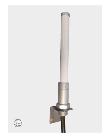
The Xbeam<sup>™</sup> XL EX is an ATEX and IECEx approved RF antenna for creating wireless networks (typically Wi-Fi, ZigBee, Wireless HART and ISA100) and wireless telemetry systems in hazardous area. The antenna is not limited to a specific network protocol and can be used for any 2 - 6 GHz application. The antenna is optimized for use in steel and concrete structure environments where multipath effects and reflections are present.
