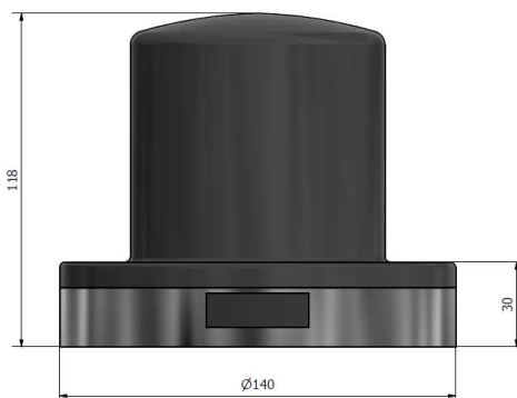
Fig 2. Physical dimensions of the Xbeam™ LTE EX Antenna (approx. dimensions in mm).
