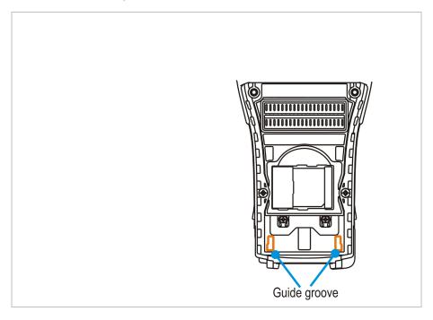
7. Snap on the keypad in the direction (see following illustration) of the arrow and push it upwards until the boreholes for the screws are over the threaded sleeves.
