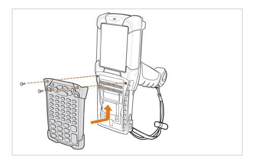
8. Check that the keypad is mounted correctly.
