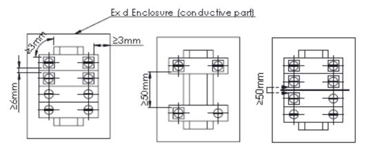
The content of the DE8-BC enclosures may be placed in any arrangement provided that an area of at least:
