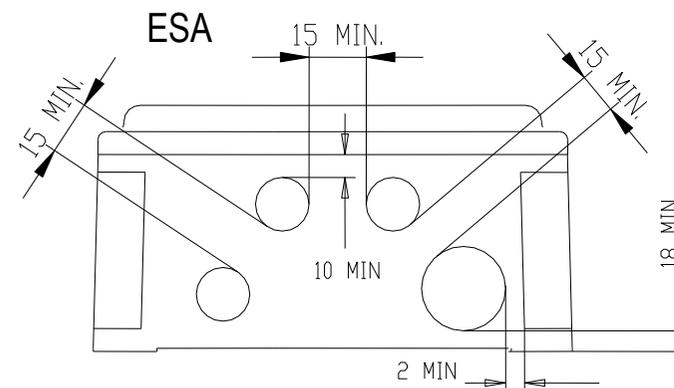
Cables entry must be carried by cable glands in case with of adapter.
