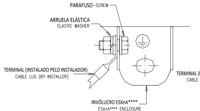
PARAFUSO ADEQUADO PARA TERMINAL DE APERTO PARA CABO 4mm2
