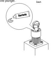
3. Release the retaining ring carefully. Take care that the retaining ring is not twisted and that the retaining ring properly locks into place in the roller plunger.
