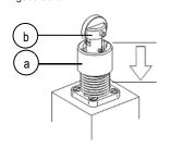
2. Apply a thin film of "BARRIERTA L55/2" lubricant (manufacturer: Klüber lubrication, material no. 090013) along the entire circumference between the top edge of the bushing and the plunger.
