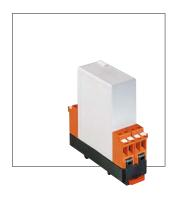
This optocoupler provides for a safe galvanic isolation between a non-intrinsically safe input circuit (transmitter) and the output connected to an intrinsically safe circuit (receiver), which is clearly identified by means of light blue terminals. The two channels are also safely galvanically isolated from each other.
