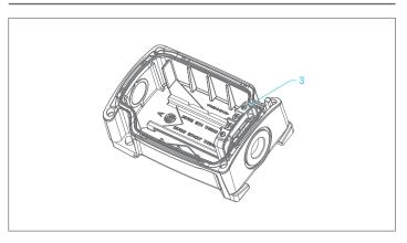
Insert the PE support (3) for the PE conductor connection either in the upper or lower area of the enclosure.
