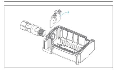
Insert the grounding plate (4) for metal cable entries between the bar and the inner wall of the enclosure. The grounding plate is secured by screwing in the cable entry.
