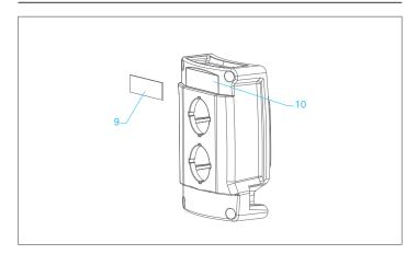
Engrave or manually label the labelling plates (9). Glue the labelling plates into the recess provided in the enclosure cover (10).
