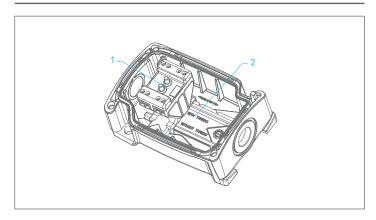
Snap the ComEx modules onto the mounting rail of the enclosure so that the detent lug is positioned in the recess of the mounting rail. Please see also the operating instructions for the individual modules.
