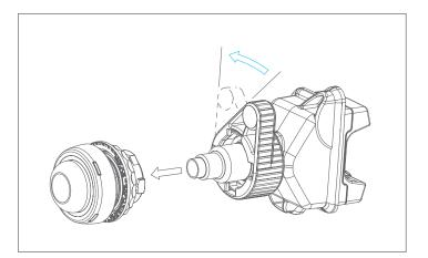
Mounting the ComEx illuminated push button module for railmounting:
