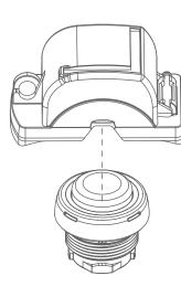
Attach the holding frame of the locking device to the actuator from above.
