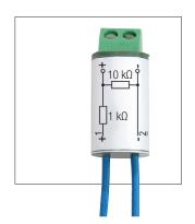
Neither can be distinguished between open circuit and open contact. This problem can be solved by installing a resistor combination at the end of the sensor line immediately before the switch. This combination provides a closed-circuit current even when the contacts is open. At closed contact it restricts the current to a value which lies clearly below the response threhold for short circuit.
