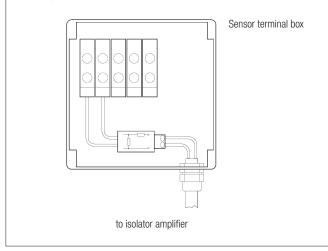
The resistive coupling element is used to monitor open and short circuits in isolator amplifier circuits controlled by mechanical contacts. The coupling element is installed directly to the control contact or inside its terminal box.
