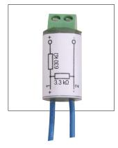
Neither can be distinguished between open circuit and open contact. This problem can be solved by installing a resistor combination at the end of the sensor line immediately before the switch. This combination provides a closed-circuit current even when the contacts is open. At closed contact it restricts the current to a value which lies clearly below the response threhold for short circuit.
