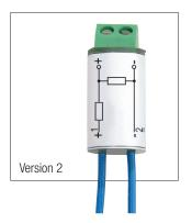
The resistive coupling element is used to monitor open circuits/short circuits on isolation amplifiers that are controlled by mechanical contacts. The resistive coupling element is installed on site directly on the contact to be monitored or in the connection area for it.
