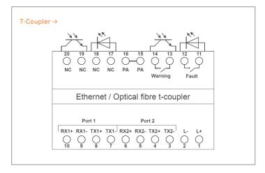
The use of 4-core Industrial Ethernet / Profinet cables is recommended, because there are no unused wires after connecting.
