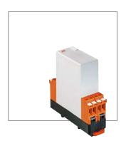
The PROFIBUS Interface terminator is an active bus terminator. Its essential benefit is the fact that bus devices can be switched off, removed or replaced without impairing data transfer. This especially applies to bus devices on both ends of the bus line through which terminal resistances previously had to be switched and supplied.
