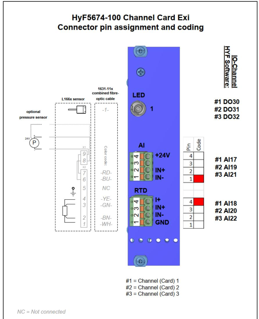
Figure 5-1: Channel card connector coding
