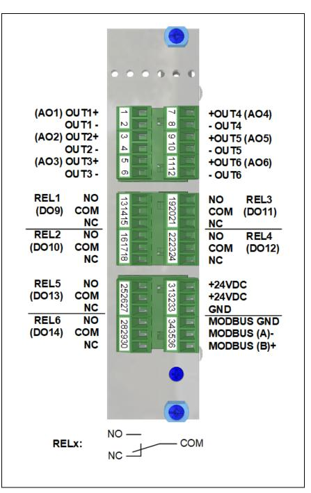
Figure 5-2: Relay connection card pin assignment
