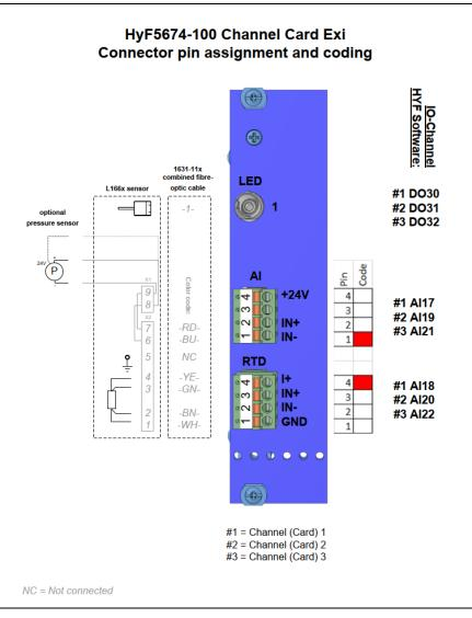
Figure 5-1: Channel card connector coding
