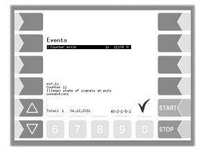
If an error occurs which prohibits a measured delivery, the pump will be disabled. The delivery must be finished.
