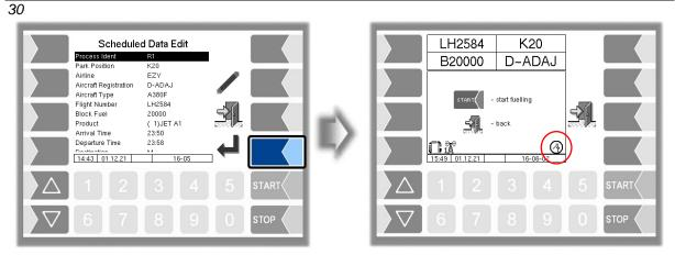
Automatic meter selection is deactivated by jumping back and the operator can select the meter manually.
