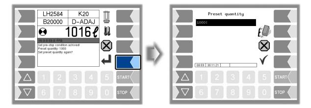
The new preset quantity is added to the current amount. Upon reaching this amount, the pump stops again automatically.
