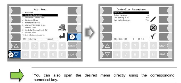
If the menu contains further submenus, you can open the required submenu in the same way.
