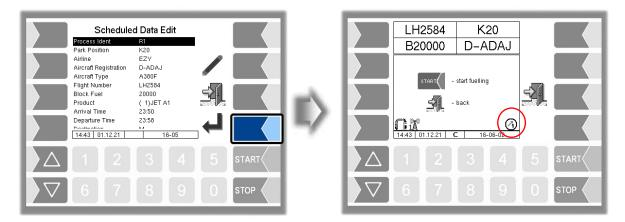
If a transaction type is selected which has no meter assigned to it, e.g. TU or RB, then you must select the meter manually.
