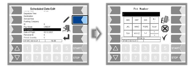
If several fuelling stations are available in a parking position, it may be necessary to supplement the information on the parking position.
