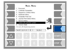
You can switch off the system properly via the main menu, the start screen and the special functions in the tour.
