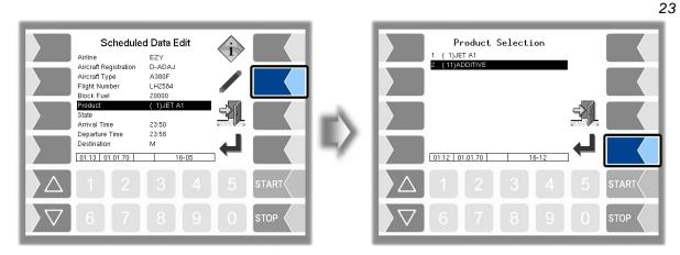
If an additive product was selected in the order function and a meter other than meter 1 was then selected in the "Select Meter" window, no delivery can be started; the "Start delivery" softkey is not displayed.
