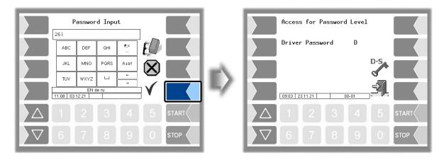
You can use the softkey to reopen the window to enter the password (driver, user or service password). Leave the password entry using the "Accept and save" softkey. After leaving the main menu, you must enter the password again.
