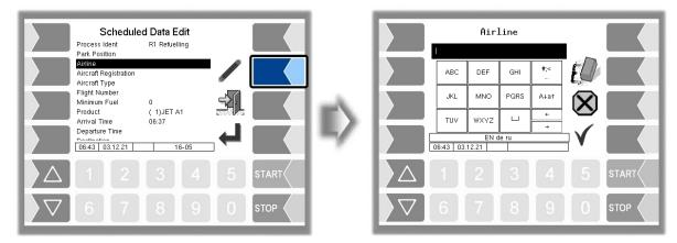
To enter the name of airlines you can use the internal database as input help.
