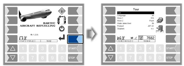
For the shift start or the driver registration the RFID TAG must be used. To do this, the operator/driver must hold the RFID TAG in front of the TAG reader. The system uses the pre-installed driver database to check the validity of the RFID TAG. If the login is successful, the ID of the operator (in the "Tour" window) and the "Confirmation" softkey will appear on the display.
