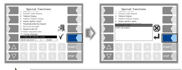
If the system is switched off via the "Special functions" window, the tour/shift will not be ended.
