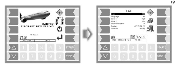
Successful registration also corresponds to the start of a tour. The driver-ID will be included in the tour journal. The tour will end when you switch to the "Start screen/main menu" window. If a change in driver is detected during a tour, the current tour will end and a new one will start. During a break, for example, you can also switch off the controller system via the "Special functions" window without leaving the tour.
