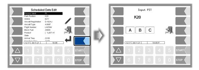
Enter the PIT number directly to select the connection point. The PIT number designation is then added to the parking position. You can only switch to the next window after you have selected the connection point.
