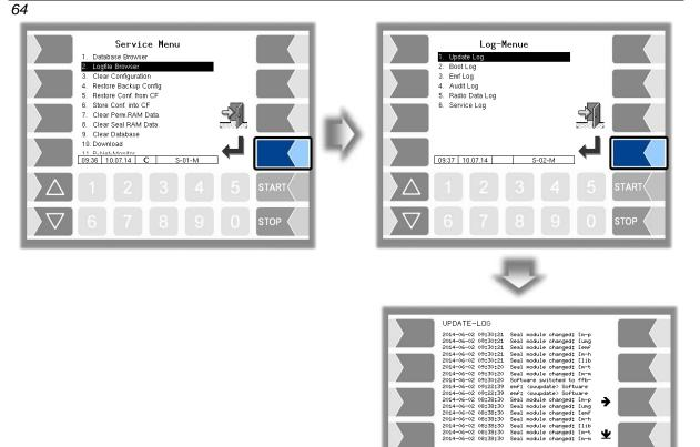
Within the log window, you can move the displayed content to the left, right, up or down using the arrow softkeys.
