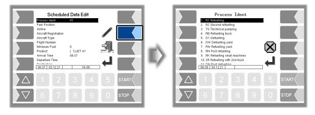
Different types of processes are available, depending on the vehicle configuration. The number of selectable process IDs is also different for Refuel- and dispenser vehicles (Configuration: Sequence Controls Menu/ Truck Parameters/Users)
