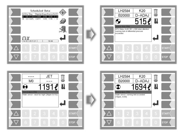
If an error occurs during an active delivery, causing this delivery to be interrupted, the event display window containing the relevant error message appears for 20 seconds.
